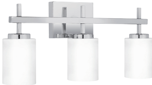
WLB8613C 10" H x 13" W x 5.75" D Finish: Polished Chrome Integrated LED Lumens: Delivered 1050 | Initial 1400 Kelvin 3000, CRI 90 ETL Listed Location: Damp (NOT TO SCALE)
